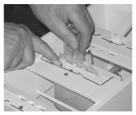
Push START to begin thawing for the programmed time. The RACK will slide back and forth forcing the plasma bags against the rods of the RACK and massageing the plasma. Use PLUS or MINUS to increase or decrease the thawing time. When the time is finished, the buzzer will call the operator back.
